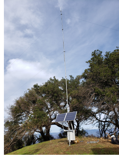
Figure 5: Solar-Powered LoRaWAN gateway at the Pepperwood Preserve deployment
